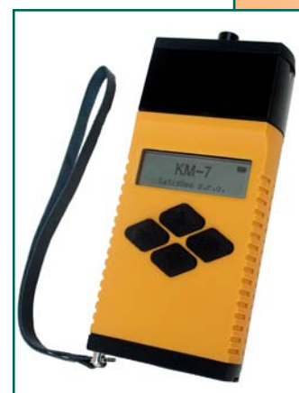
KAPPAMETER KM-7 Pocket Magnetic Susceptibility Meter
