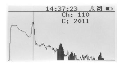
Identification and analysis of small peaks can be performed by the change of the vertical scale by means of push-buttons [ $\land$ ] and [ $\lor$ ] multiplying or dividing the scale by a factor of 2. This can be repeated several times. Contents of channels, whose value exceed the vertical scale, do not change and remain of its value, surpass the upper limit of counts of displayed spectrum, and do not disturb the graph of small peaks.
