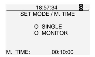
Measurement mode can be selected by means of keyboard push-buttons
