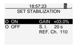
The automatic digital spectrum stabilization can be switched off. In that case, concentrations of K, U, Th are not calculated.
