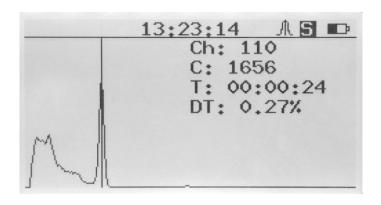
Cursor is marked in the displayed spectrum by a vertical line and can be shifted horizontally by push-buttons [<] and [>]. If the push-buttons [<] or [>] are kept pressed, the cursor movement is accelerated. The last cursor position is retained in the memory and will be applied in the next measurement.
