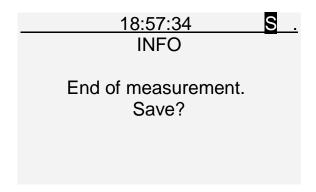
The data are saved by pressing the push-button [ENTER] or not saved by pressing the push-button [ESC], and the control returns to the main menu.
