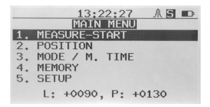
The backlight is switched off automatically 10 seconds (default value is 10 s, other options selectable) after the last pressing of a push-button. The backlight can be switched off all the time to save power consumption. (See the item 4. BACKLIGHT of the setup - system menu.) The first icon in the upper right corner of the screen indicates that stabilization is on, the letter S means mode SINGLE is set (M stands for MONITOR), the last icon indicates status of batteries.
