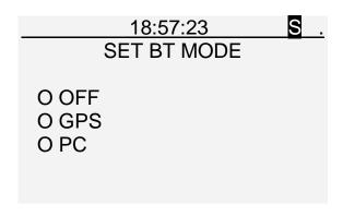
The instrument can communicate with the GSP receiver or with a PC. However data transfer to a PC via Bluetooth is much slower than via USB and usually is not used.
