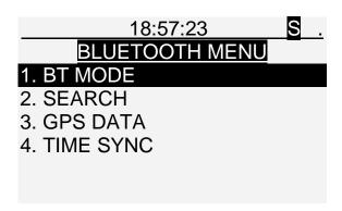
Activating item 1. BT MODE displays radio buttons to select the BT mode. Default value (after switching the instrument on) is OFF.
