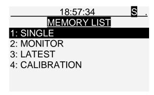
After selecting an item and pressing [ENTER] the display shows information: "No single measurement." (e. g.) if there are no data of the desired type, and a list of measurements if there are any in the memory.
